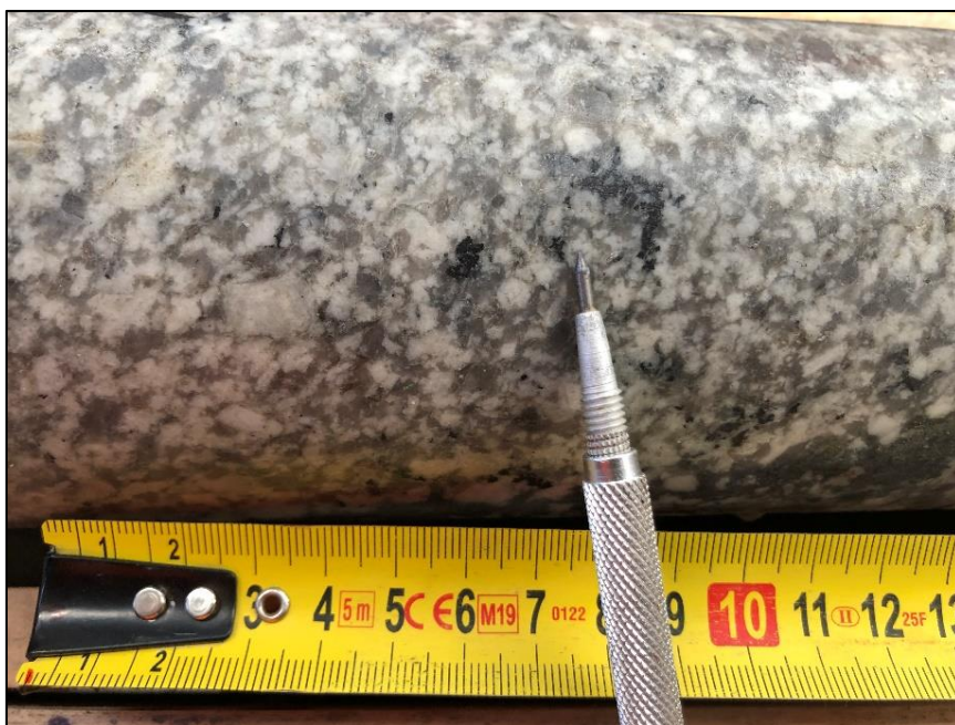
Figure 4. Endogranite with clusters of millimetric crystals of disseminated wolframite and minor cassiterite (21DD0008, 68.40m). This sample returned 0.22% WO 3 and 558ppm Sn over 3.00m.
